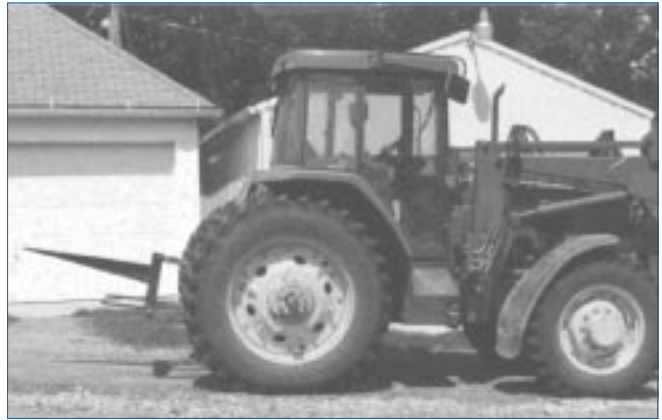
Photo 2. The tractor shown in the photo has a rear-end bale spear attachment. Moving the bale with the rear end bale spear attachment makes the tractor more stable, does not get in the way of the tractor's headlights, and allows the operator a clear view.
