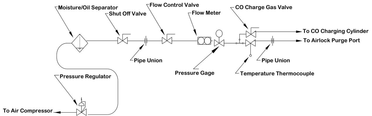
Figure 8. Purge plumbing diagrams. Top diagram is for the tent-type refuge alternative airlock. Bottom diagram is for the rigid steel refuge alternative airlock.
