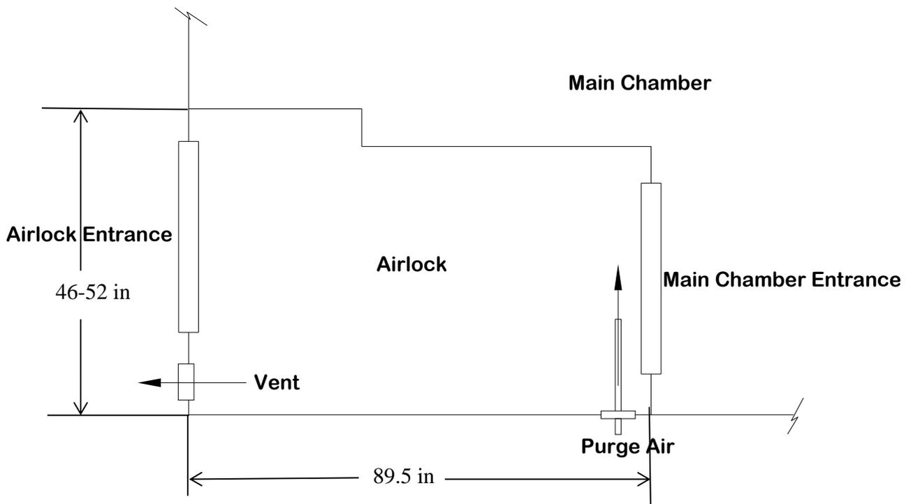
Figure 7. Plan view of air flow schematic for the rigid steel refuge alternative airlock during purging.
