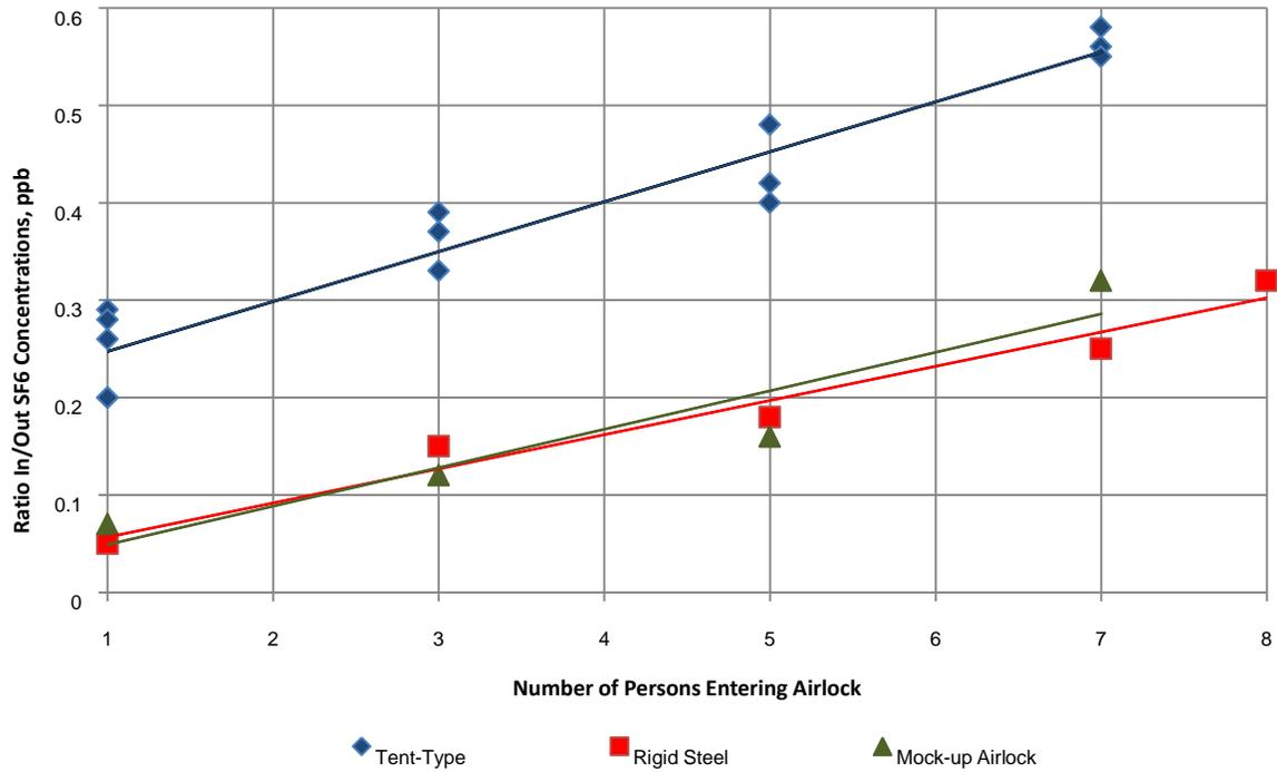
**Figure 17. Graph of the ratio of SF<sub>6</sub> concentration (surrogate for carbon monoxide) in the airlock and outside the airlock versus the number of subjects entering the airlock (from data in Table 13).**
