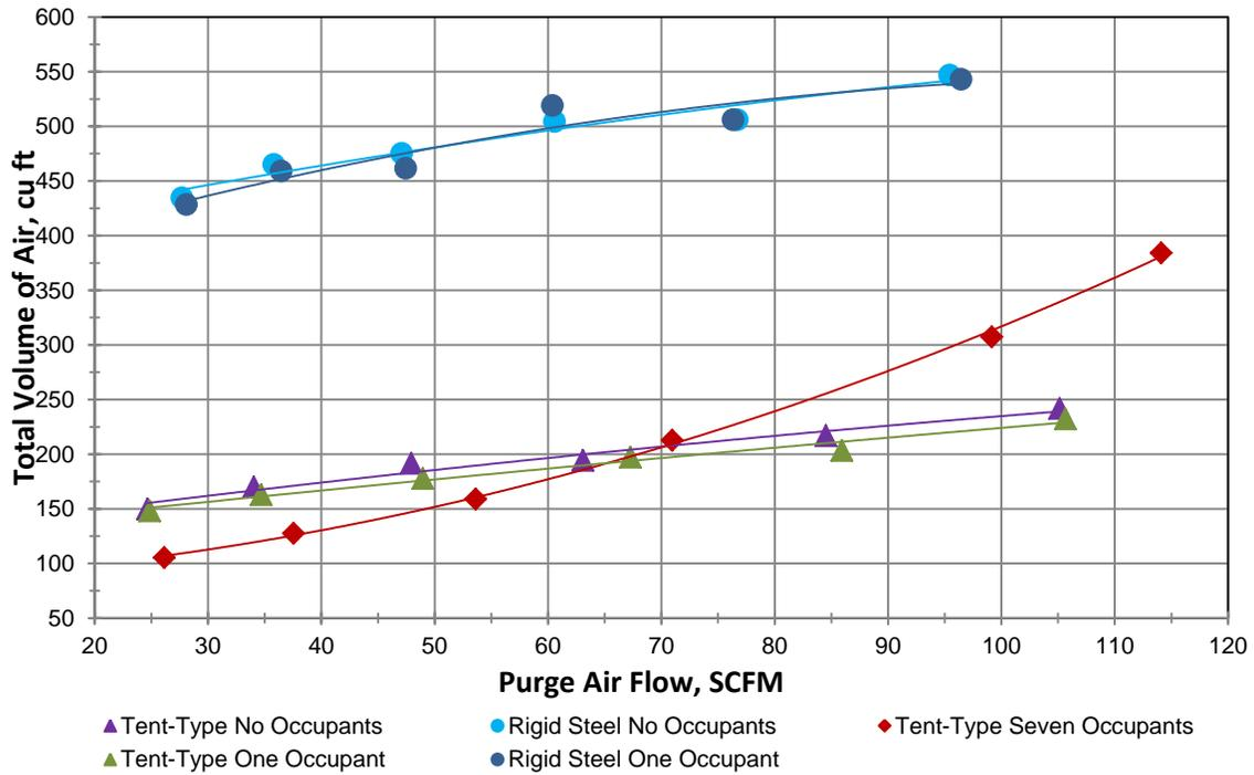
Figure 12. Graph of total volume of air required to purge versus air flow rate.
