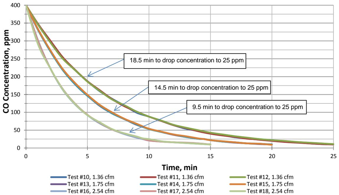
**Figure 3. Mini purge box test results at 0.13 psig relief pressure and three different purge air flow rates.**
