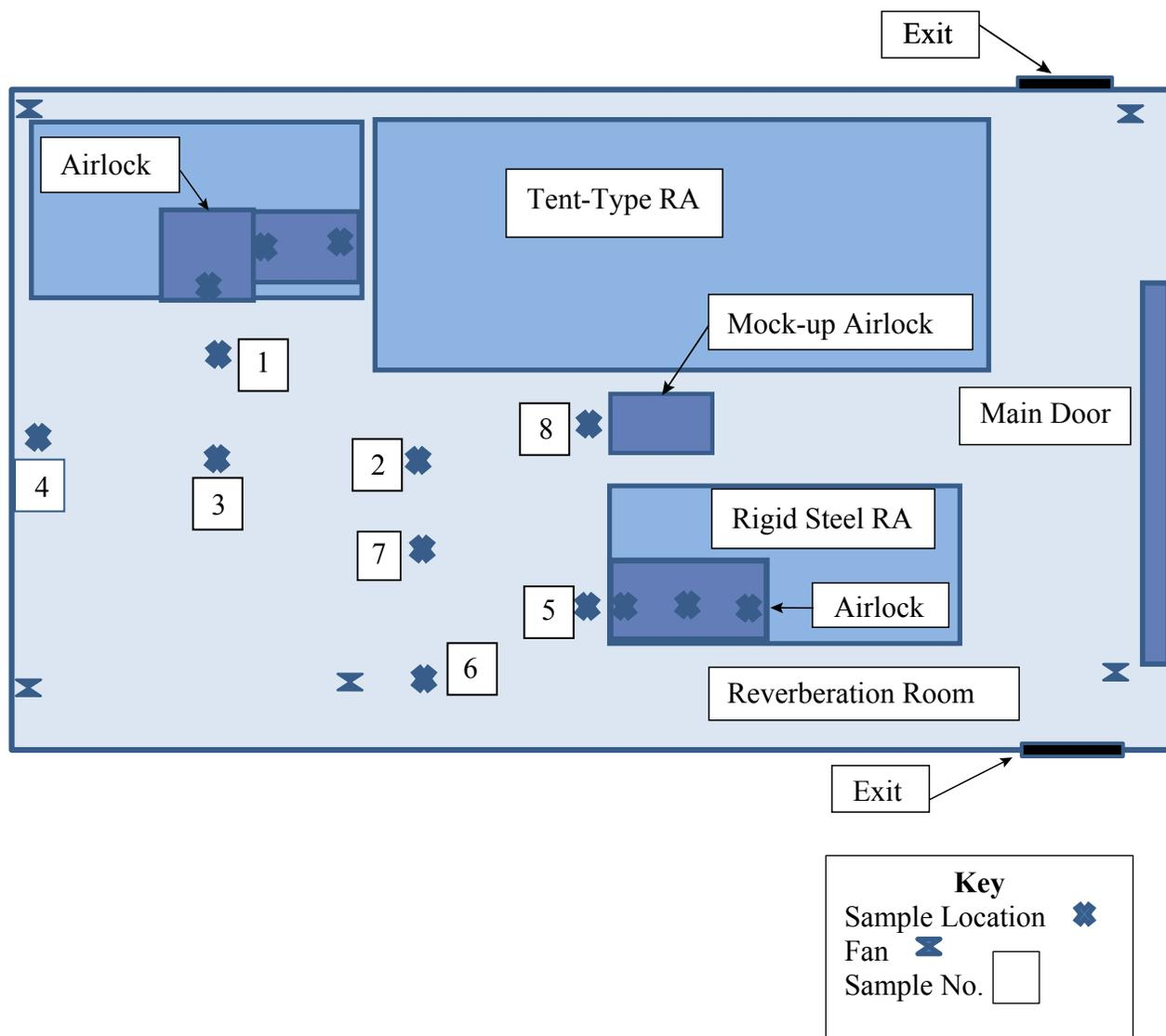
**Figure 16. Reverberation room showing mobile refuge alternative locations, fan locations, and sample recording locations. Sample locations 1, 2, 3, and 4 are for tent-type refuge alternative airlock test, locations 5, 6, and 7 are for the rigid steel refuge alternative airlock test, and location 8 for the mock-up airlock tests. Note: Drawing is not to scale.**
