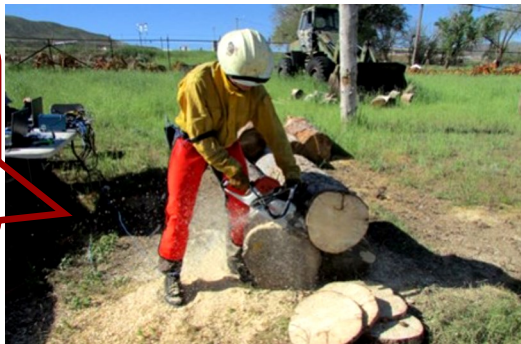
Sawyer cuts slices from logs while the vibration is measured at the hand-handle interface. Photo by NIOSH.
