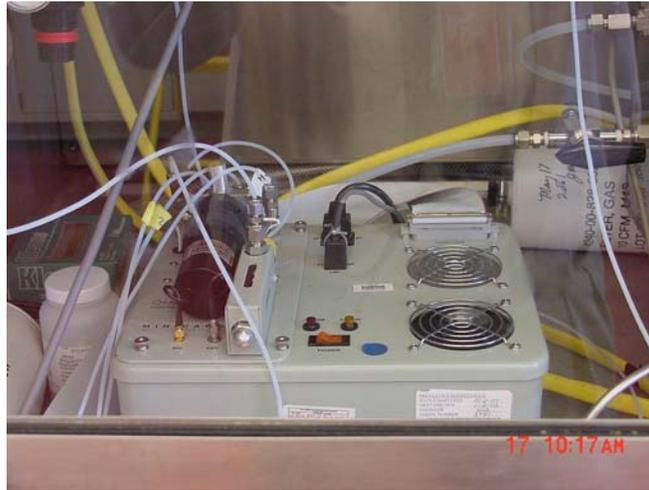
**Picture 3: Miniature Continuous Air Monitoring System, (MINICAMS)**
