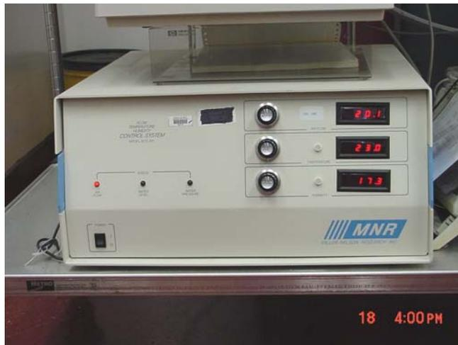
**Picture 5: Flow-Temperature-Humidity Control System**
