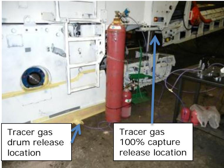
Figure 3: tracer gas injection locations
