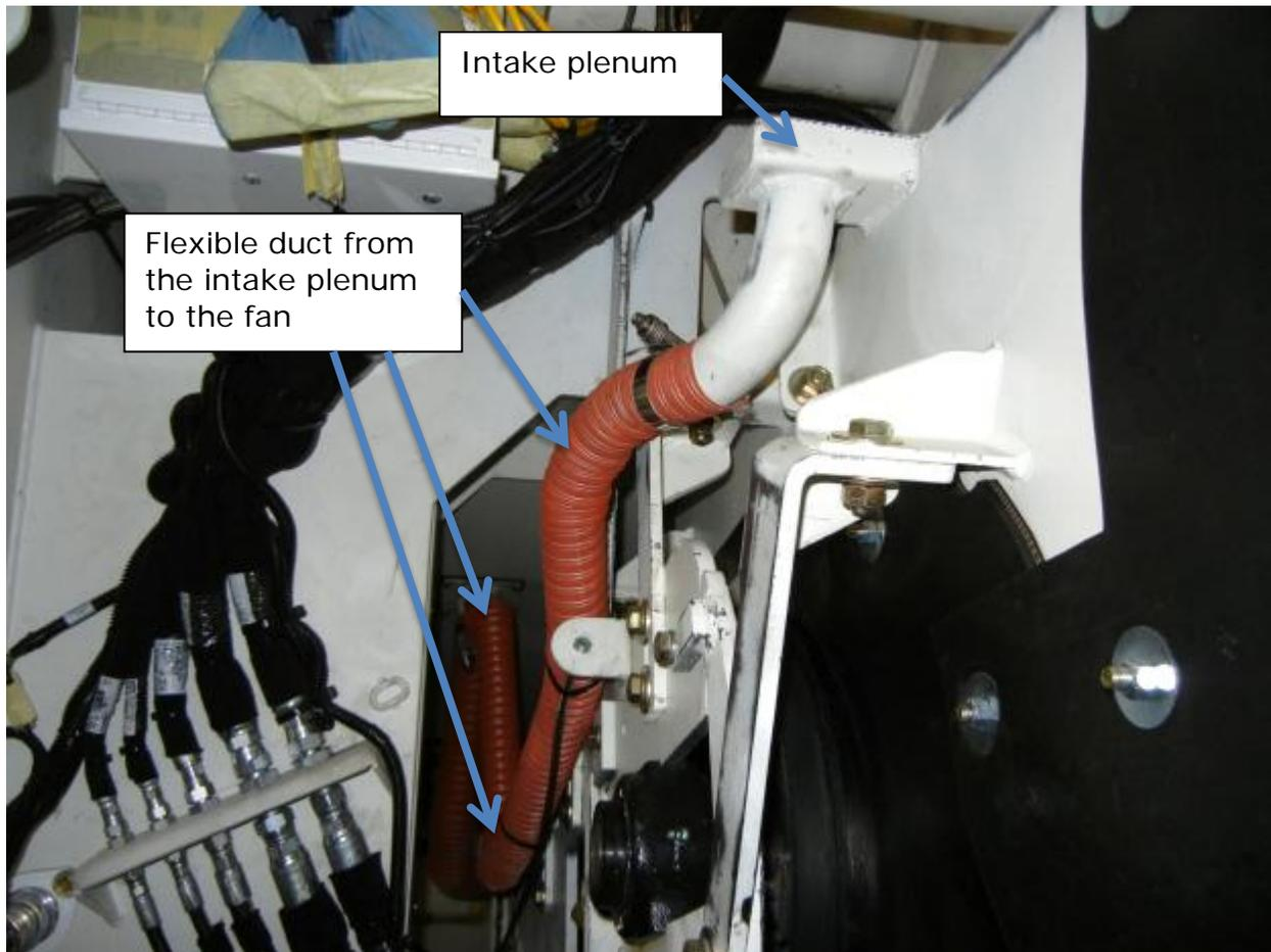
Figure 7: Flexible duct on the suction side of the fan
