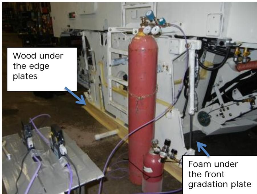
**Figure 1: Wood, tape, and foam used to fill in gaps.**
