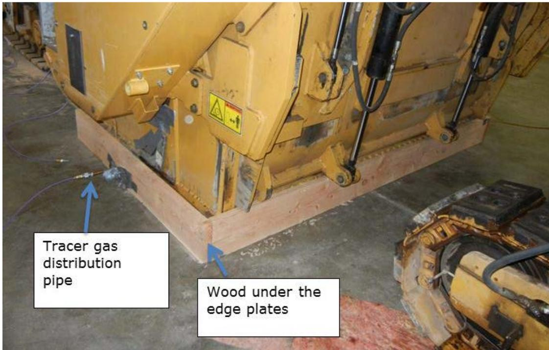
Figure 1: Wood used to fill in gaps for test.
