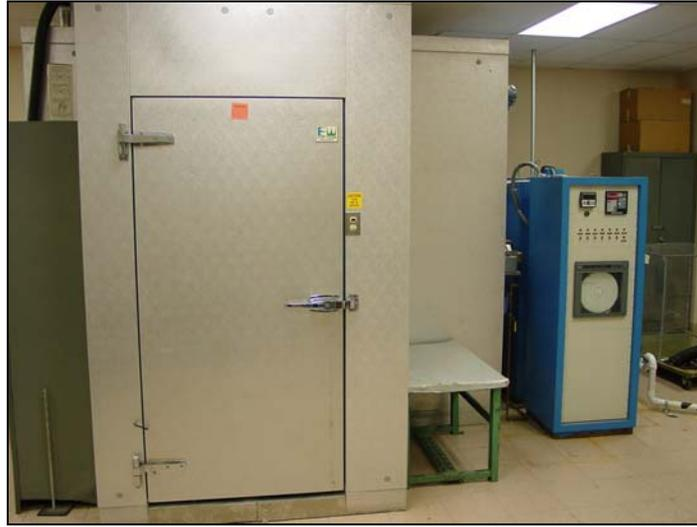
**Figure 2. Environmental Walk-In Chamber, Model D69 manufactured by Tenny Engineering, Inc.**
