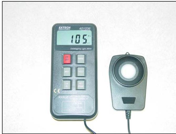
**Figure 4. Light Meter, Model 401036, by Extech Instruments**
