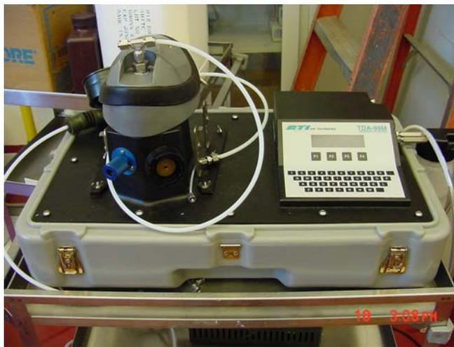
**Picture 2: Respirator Leak Detector, Model TDA-99M**
