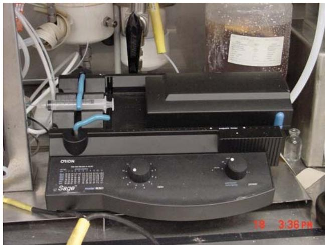
**Picture 4: Syringe pump, Sage Model M365**
