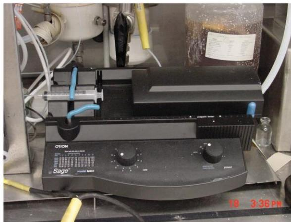
**Picture 4: Syringe pump, Sage Model M365**
