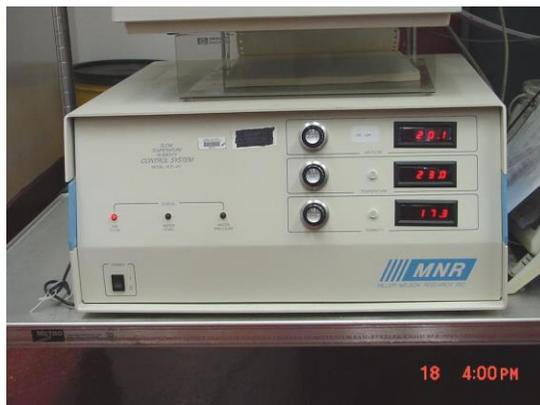
**Picture 5: Flow-Temperature-Humidity Control System**
