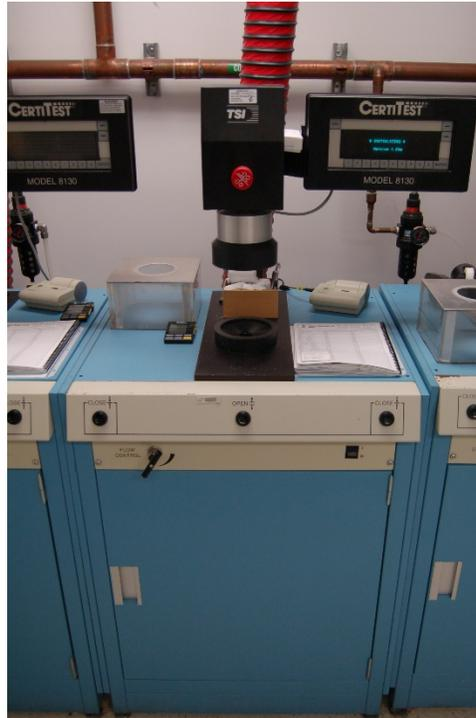
8.3. Close-up of respirator test fixture with the chuck closed
