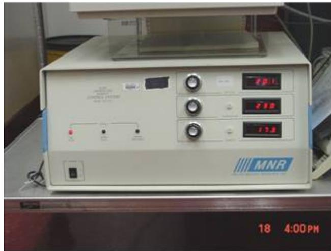
**Picture 5: Flow-Temperature-Humidity Control System**
