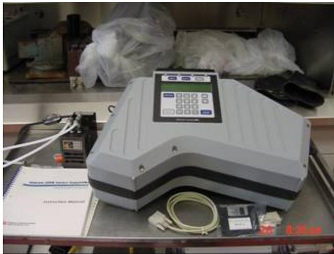
**Picture 9: Miran Analyzer, Model 1A**
