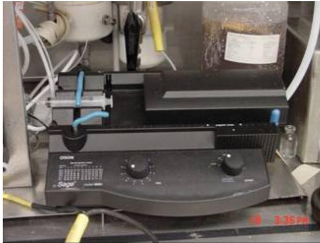
**Picture 4: Syringe pump, Sage Model M365**
