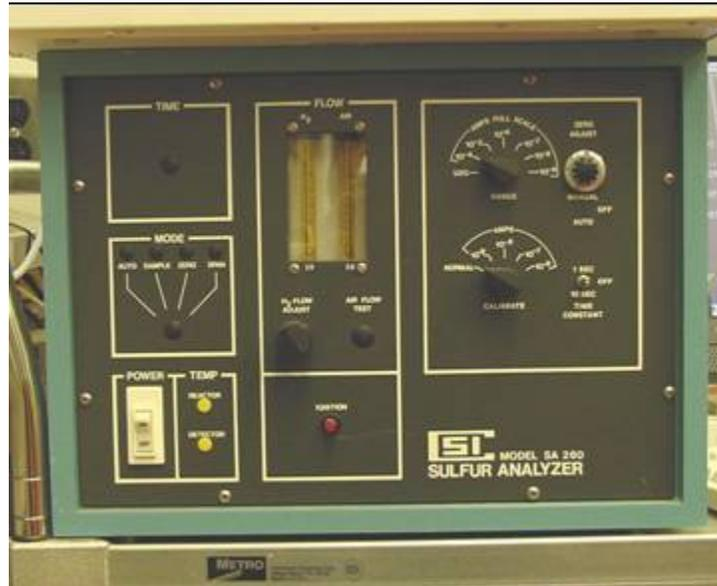
Picture 9: Hydrogen Flame Emission Detector (HYFED), Model SA 260
