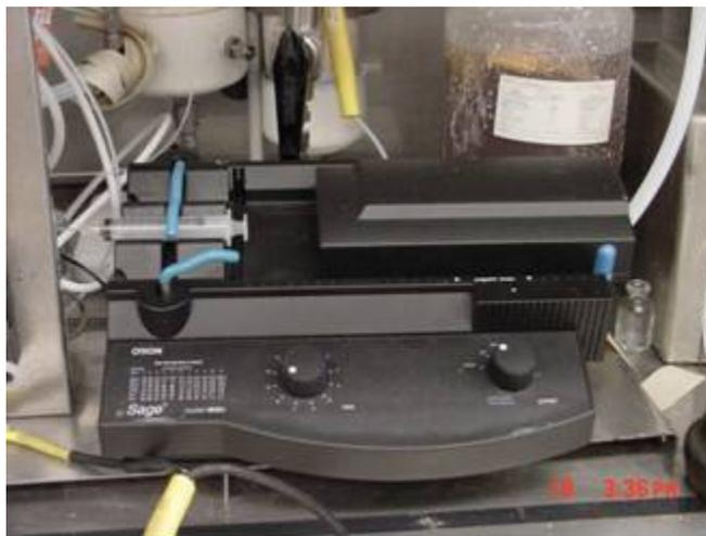
**Picture 4: Syringe pump, Sage Model M365**
