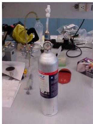
3.1.4. Nitrogen dioxide certified gas cylinder, 1 ppm  $\text{NO}_2$ , balance gas helium with 3510-660 regulator.
