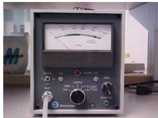
3.1.2. Interscan Corporation Model 1152 Nitrogen Dioxide Analyzer or equivalent.
