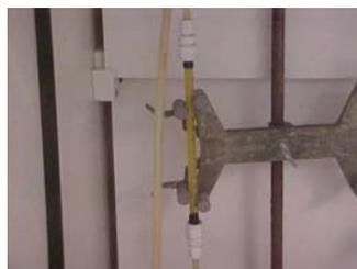
3.1.5. Brooks Rotameters, R 215-D for cartridges or mass flow controller, 0-50 ml/min.
