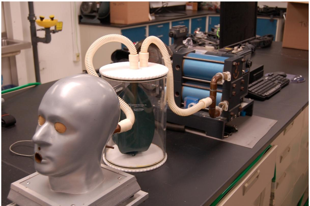
Figure 1: Flow Rate Determination Breathing Machine Set-up
