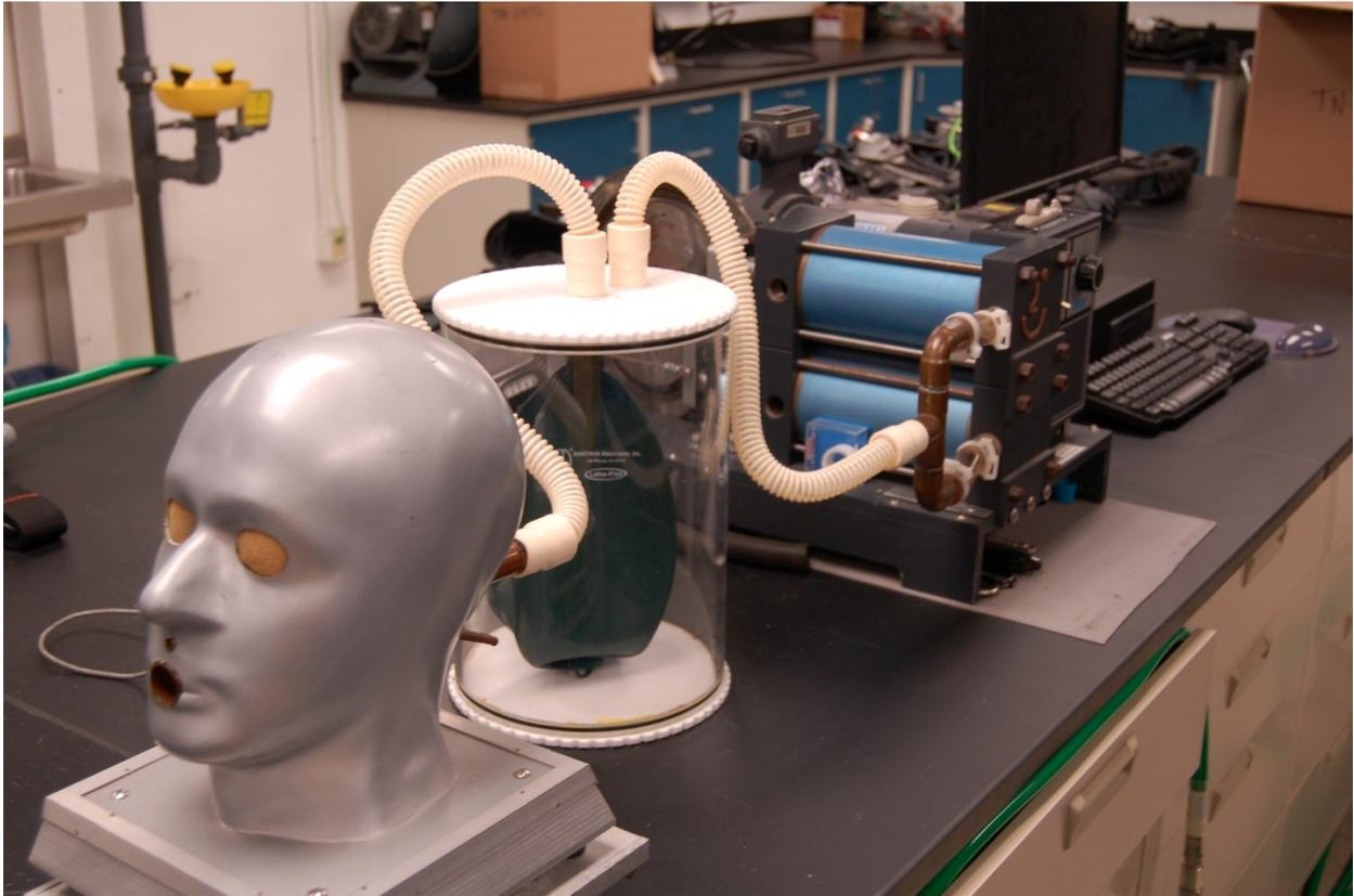
Figure 1: Breathing Machine Set-up
