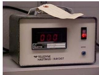
3.1.1. Teledyne Hastings - Raydist Mass Flow Meter - Model NAHL-25 or equivalent.
