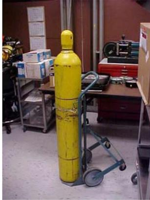
3.1.6. A 300 cubic foot gas cylinder of compressed air or equivalent.
