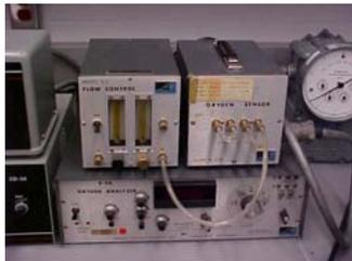
3.1.9. Applied Electrochemistry Oxygen Analyzer - Model S-3A or equivalent.
