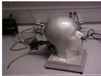
3.1.1. ISI Anthropometric Test heads with tube for measuring breathing resistance and air flows - Model SR-085 or equivalent.
