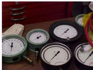
3.1.1. Helicoid calibrated test gauges, traceable to NIST.
