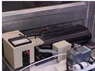
3.1.9. Infrared Analyzer Gas Analyzer (Miran/A) or equivalent.
