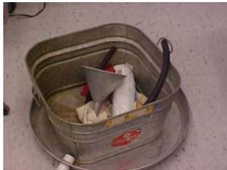
3.1.4. Large container or tub, (14" deep x 22" W x 22" L) approximately 20 to 30 gallon capacity or equivalent.
