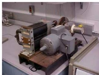
3.1.1. Mechanical Breather with 622 Kg-m/min. cam as per U.S. BOM Drawings C-1748 (3/17/69) Breathing Machine and B-1198 (3/6/69) Breathing Cam.
