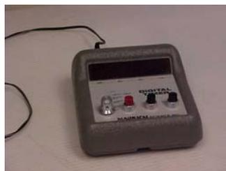
3.1.1 Electric timer, calibrated to hundredths of a minute (Precision Scientific Company).
