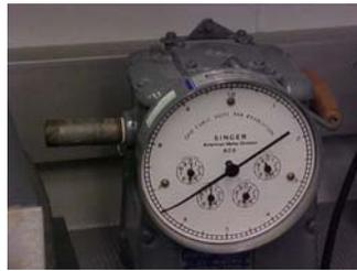
3.1.2. Dry test - Gas meter, (Singer-American Meter Division - Model DTM-200A) varies depending on expected flow.
