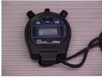
3.1.7. Timer, Digital stopwatch, calibrated to hundredths of a minute (Cronus Precision Products, Inc.) to hand carry. or equivalent.
