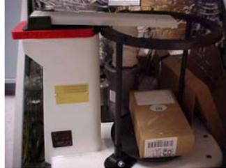
3.1.2. WS Tyler Rotap Machine - Model RX30 or equivalent.
