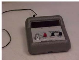
3.1.5. Electric Timer, calibrated to hundredths of a minute (Precision Scientific Co.) or equivalent.
