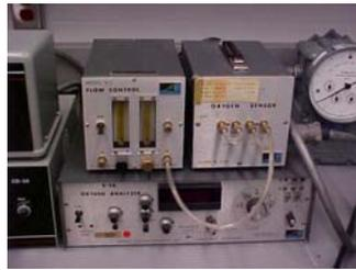
3.1.2. Applied Electrochemistry Oxygen Analyzer - Model S-3A or equivalent.
