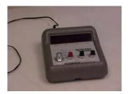
3.1.1. Electric Timer, calibrated to hundredths of a minute (Precision Scientific Company) or equivalent.
