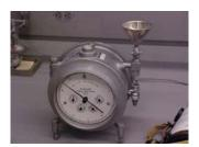
3.1.3. Wet Test - Gas Meter (Singer-American Meter Company - Model AL17-1) or equivalent.
