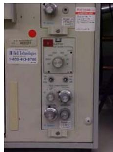
3.1.1. Two channel thermal tip recording system (Gould Model No. RS3200) with carrier amplifier (Model No. 13-4615-35) or equivalent.
