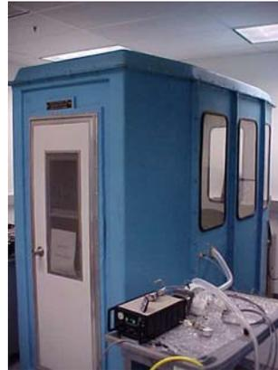
3.1.15. Corn Oil Generator and Chamber - Dynatech Frontier Enterprises Model 260 - (May be substituted for No. 3.1.8., above) or equivalent.
