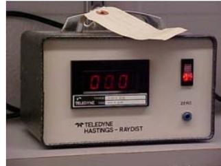
3.1.16. Teledyne Hastings - Ray Dist Mass Flow Meter - Model NAHL-25 (May be substituted for No. 3.1.13., above) or equivalent.
