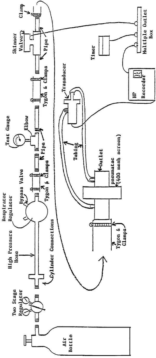
Figure 1 - Overpressurization Test Setup
