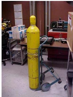
3.1.1. A 300 cubic foot gas cylinder of compressed air or equivalent.
