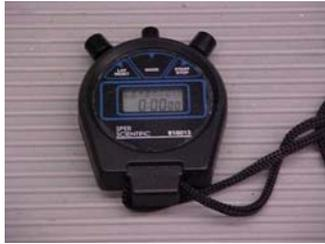
3.1.2. Timer, Digital stopwatch, calibrated to hundredths of a minute or equivalent. (Cronus Precision Products, Inc.)
