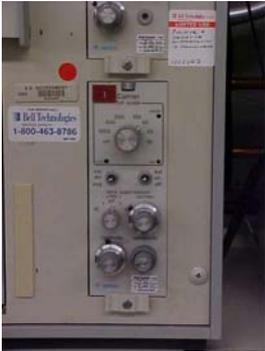
3.1.4. Two channel thermal tip recording system (Gould Model No. RS3200) with carrier amplifier (Model No. 13-4615-35) or equivalent.
