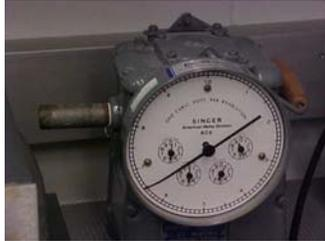
3.1.3. Singer Dry Test Meter (Model 806) one cubic foot per revolution of proper rater or equivalent.
