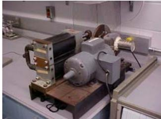
3.1.5. Mechanical Breather with 622 Kg, m/min, Cam (as per U.S. BOM Drawings C-1748 (3/17/69) Breathing Machine and 8-1198 (3/6/69) Breathing Cam.
