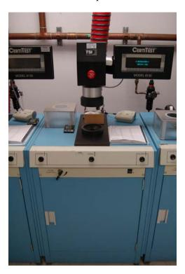
8.3 Close up of respirator test fixture in the closed chuck
