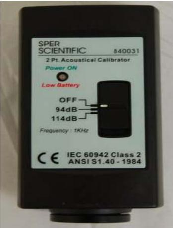
**Figure 4. Acoustical calibrator (Sper Scientific model 840031)**
