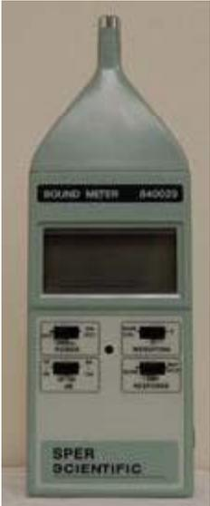
**Figure 3. Sper Scientific LTD digital sound level meter, Model 840029**
