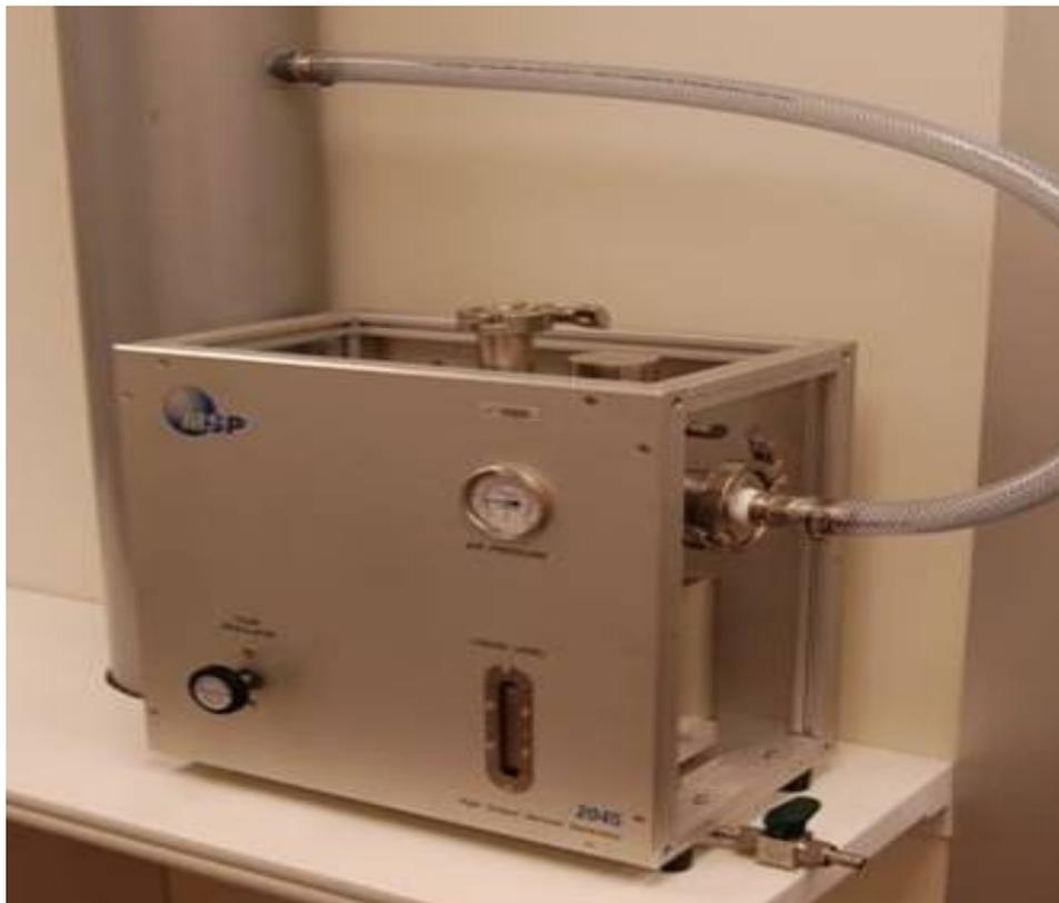
Figure 2: Aerosol Generator
