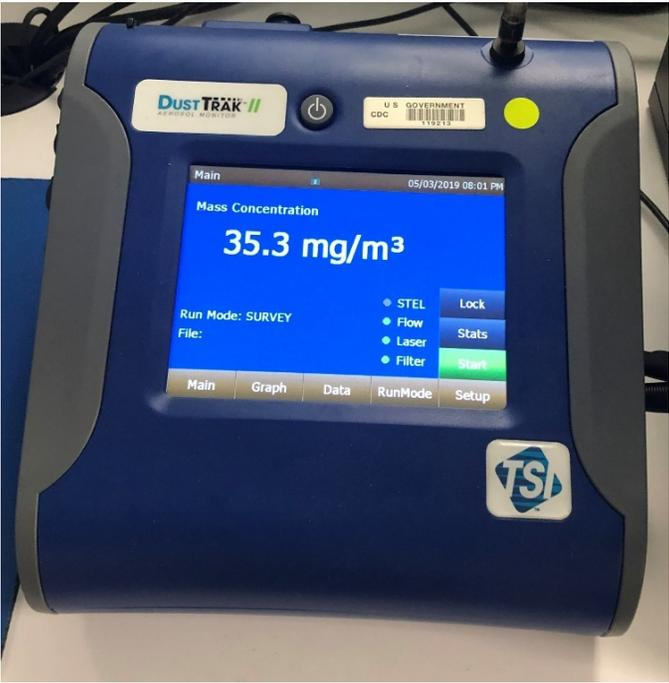
Figure 3: DustTrak II Aerosol Monitor
