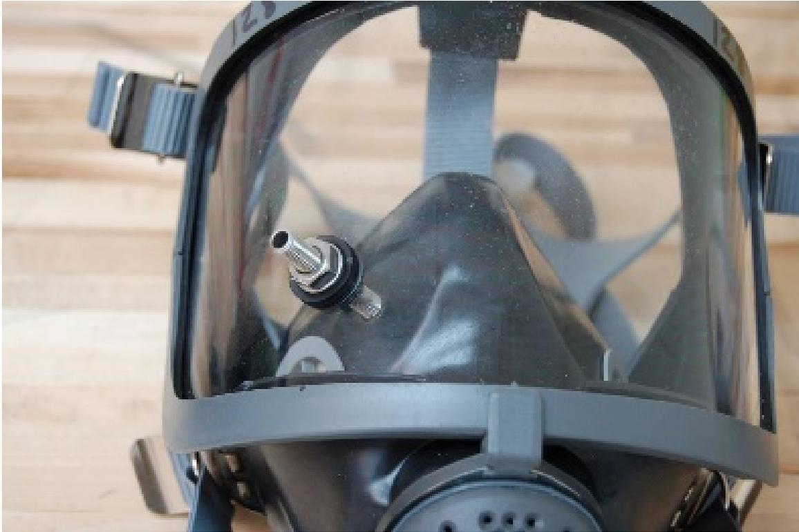
Figure 9: Exterior View of a Probed Sample Respirator
