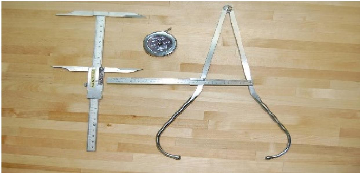
Figure 7: Facial Size Measurement Calipers
