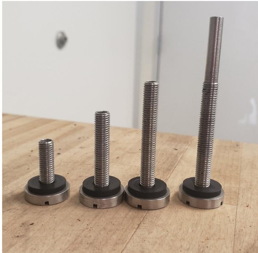
Figure 10: View of Sample Probe – Various lengths
