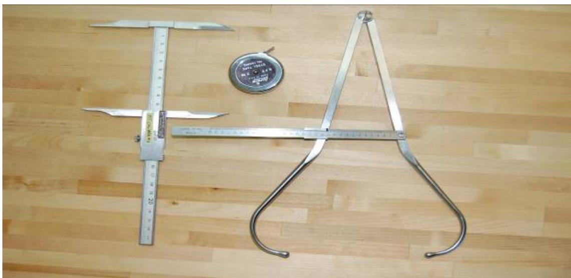
Figure 6: Facial Size Measurement Calipers
