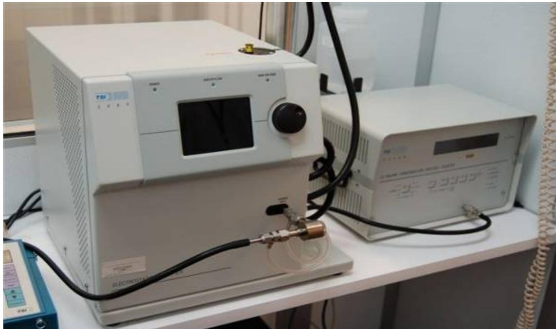
Figure 4: Scanning Mobility Particle Sizer
