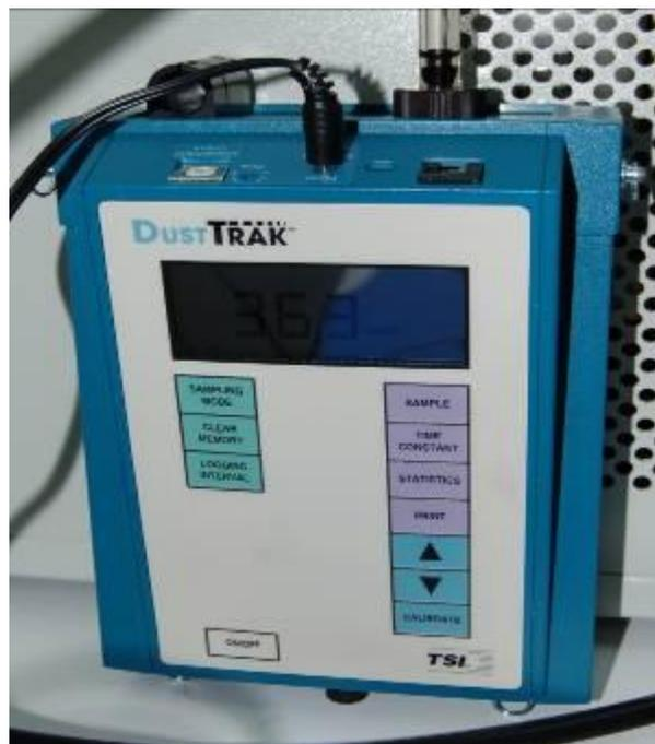
Figure 3: Dustrack Aerosol Monitor
