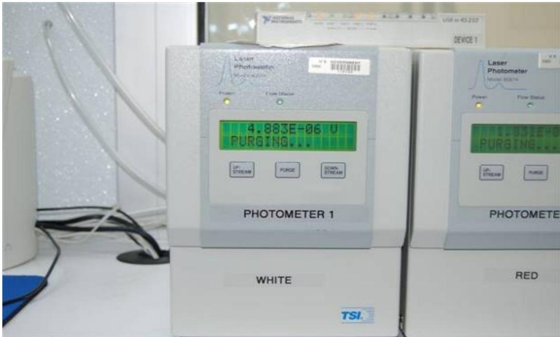
Figure 1: Laser Photometer, Model 8587A
