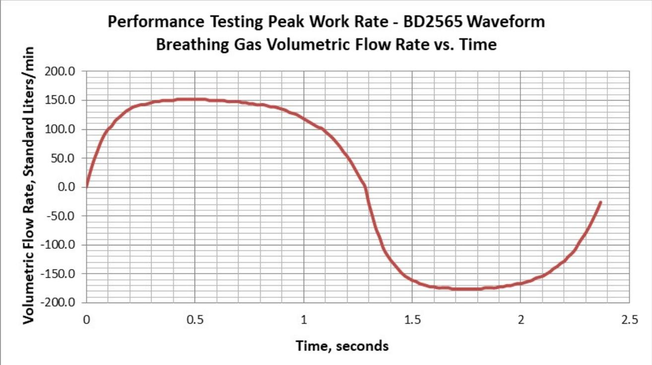
Figure 2: Example graph for Peak Work Rate, showing breathing gas volumetric flow rate (y-axis) vs. time (x-axis).
