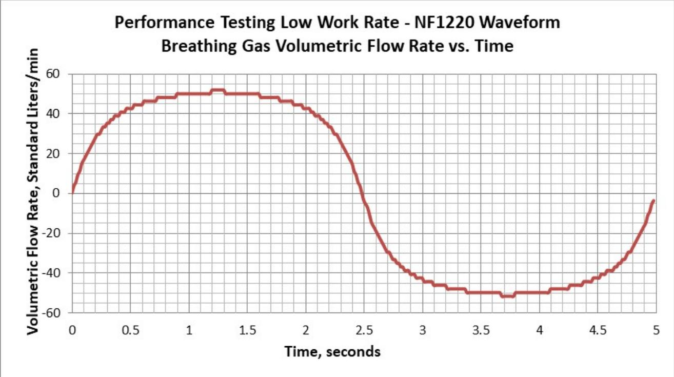
Figure 4: Example graph for Low Work Rate, showing breathing gas volumetric flow rate (y-axis) vs. time (x-axis).
