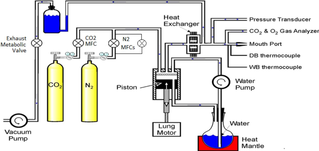
Figure 1: Schematic of the ABMS
