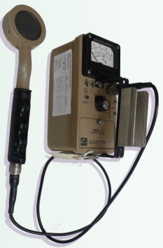
Figure 1: A pancake-style GM detector
